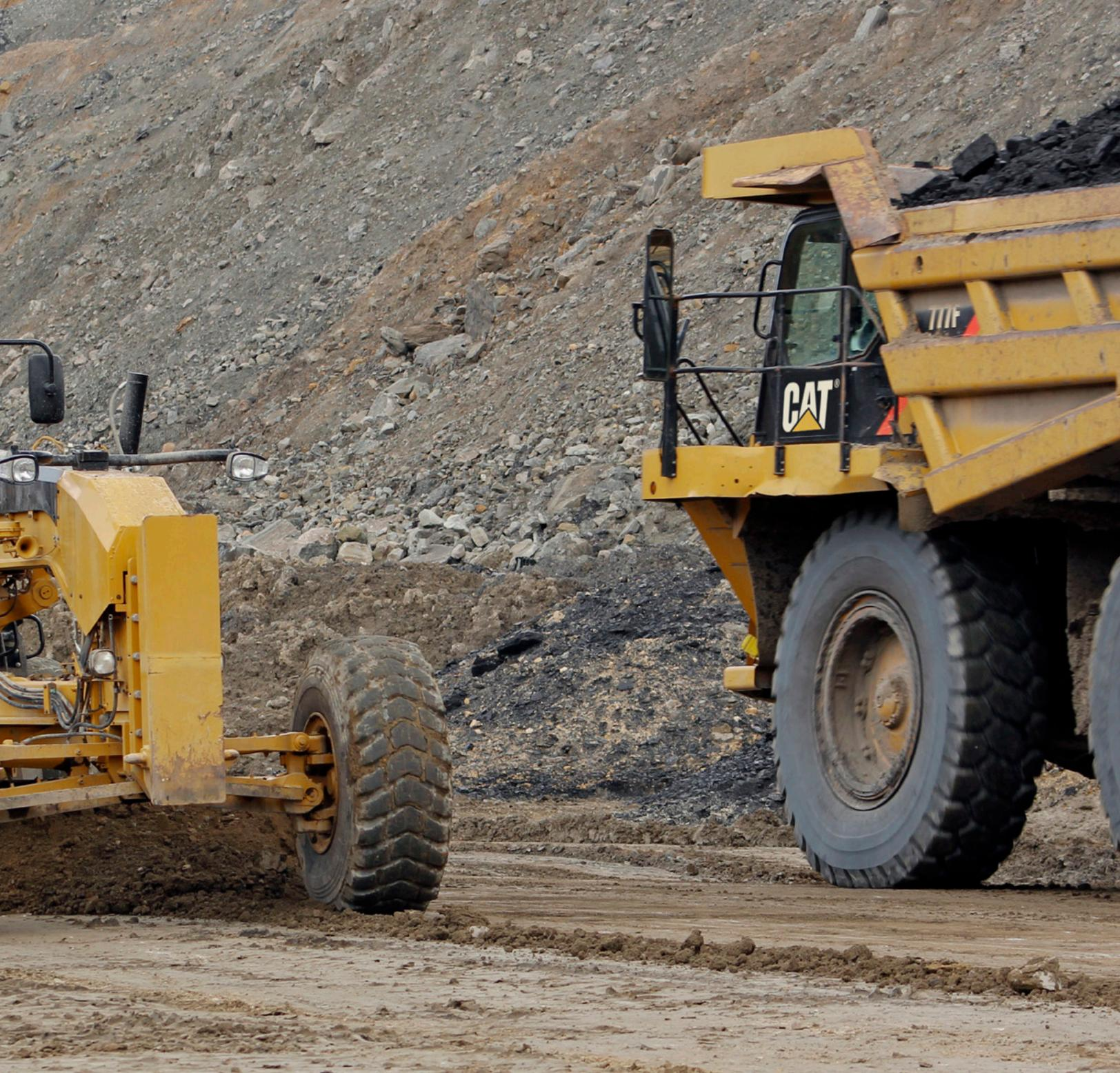
**With additional power, wider moldboard and the possibility to use a more aggressive blade angle; the 18 enhances operational efficiencies by increasing coverage and reducing the number of passes required to grade your haul roads.**
